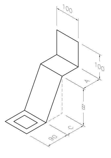
DPC Joint Support for surface fixed cavity tray with cavity insulation ledge
