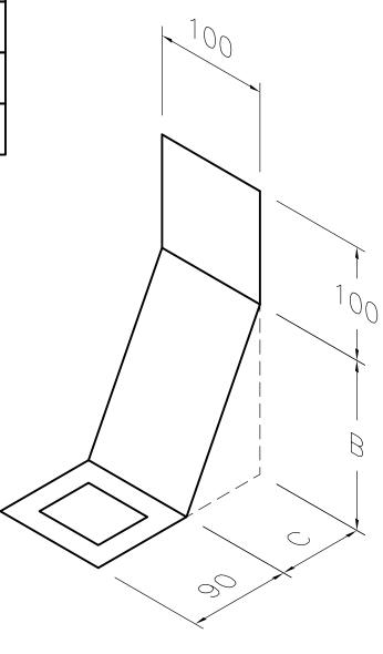
DPC Joint Support for surface fixed cavity tray without cavity insulation ledge
